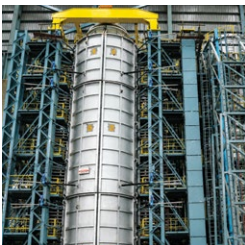
VERTICAL SHAFT FURNACE Shafts Upto: Ø 2000 mm Height: 16 meters
