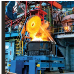
ELECTRIC ARC FURNACE (85-120 MT)
