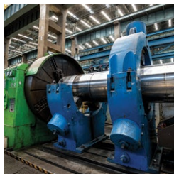
DEEP HOLE DRILLING Weight Capacity: Upto 100 MT Max. Drilling Depth: 15000 mm
