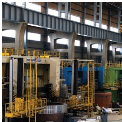
VERTICAL TURNING LATHE Weight Capacity: Upto 250 MT Max Height: Upto 5400 mm
