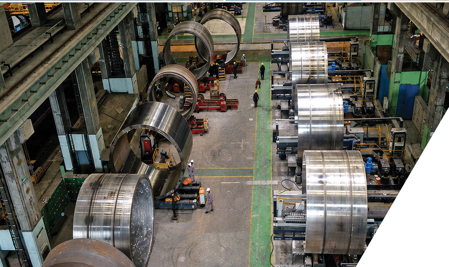
Plate-rolling machine for hot rolling of plates 300mm max. and 4500mm wide max.
