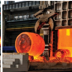
REHEATING & HEAT TREATMENT FURNACE (Upto 400 MT)
