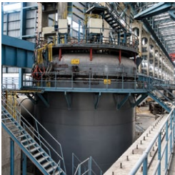
VACUUM INGOT CASTING (Upto 300 MT, H 2 <1 ppm)
