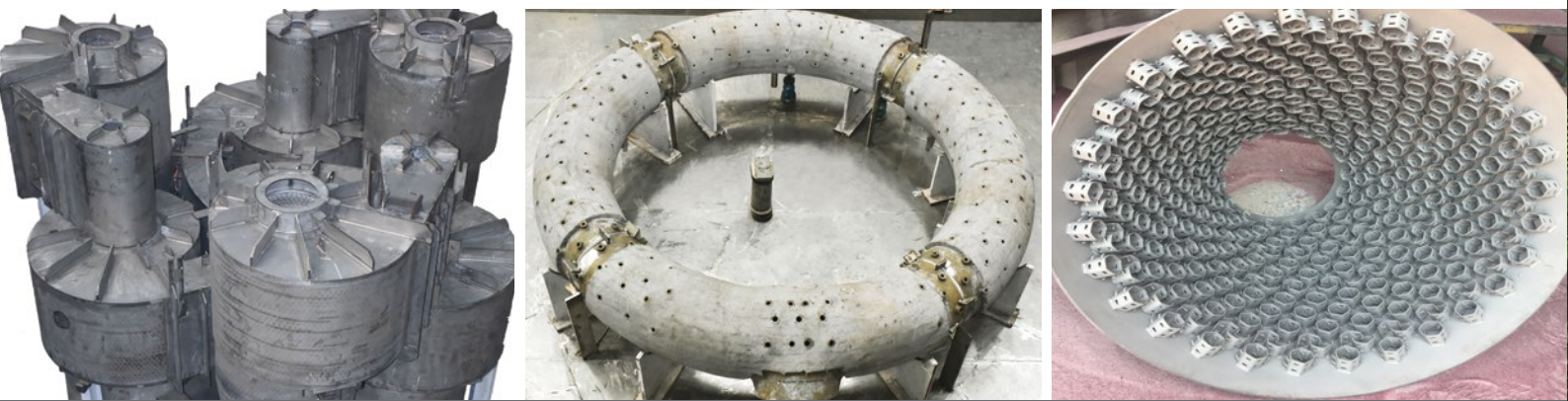
Internals for FCC - Cyclones and Air Rings
