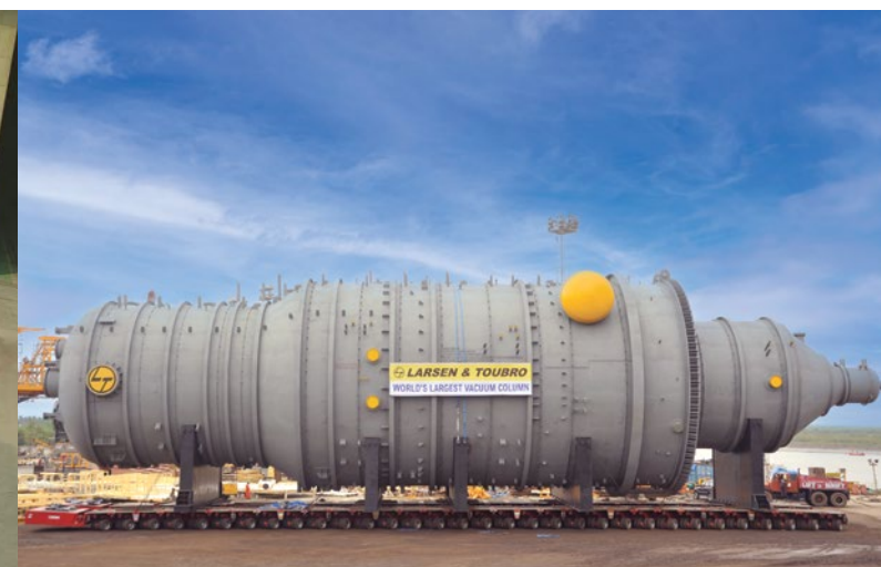
Heaviest Vacuum Column weighing 964 MT
